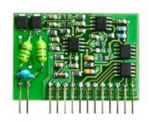
Thermocouple J (Fe-Co) input. Measuring range -200 to  $+750^{\circ}$ C. Accuracy  $\pm 0.3\%$  from reading  $+1.5^{\circ}$ C. Linearized, cold junction compensation. Galvanically unisolated.
