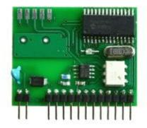
Input for measurement of frequency of voltage signal 0 to 5kHz, resolution 1Hz, accuracy  $\pm (0.2\%$  from reading + 1Hz) input voltage for state "H": 3 to 24Vdc input current in state "H": approximately 7mA minimum duration of input impuls: 30us, galvanic isolated.
