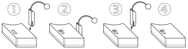
The procedure is identical with the above procedure for switching ON. If indication yellow LED does not light up to 1 second after plugging the magnet, it is necessary to unplug magnet and repeat the procedure.
