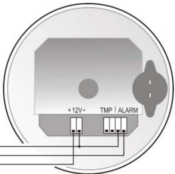
**Notice:** The connecting cables should be located as far as possible from the potential interference sources. The cable shield connect to "Shield" terminal of regulator only.
