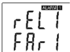
FAR0 – „far condition 0“: after device's power on the relay is open
