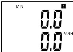
Range and type of value for output 1 ( $U_{out1}$  = symbol „1“ on display). Type of value, assigned to output 1, is indicated by displayed unit (here %RH = relative humidity). Upper line displays voltage value corresponding to measured value (lower line).
