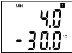
Range and type of value for output 1 (current loop II = symbol „1“ on display). Type of value, assigned to output 1, is indicated by displayed unit (here °C). Upper line displays current value corresponding to measured value (lower line). Here 4 mA corresponds to -30 °C.
