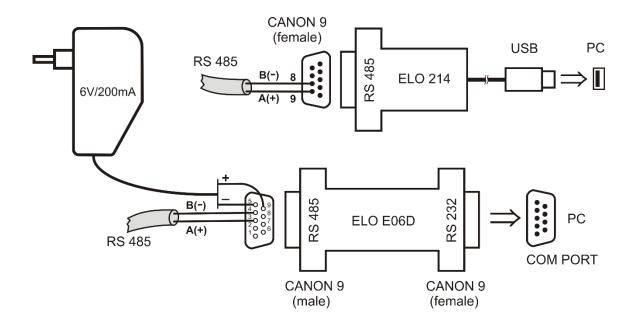
The **ELO E214** converter is an optional accessory for connection of transmitter with RS485 interface to the PC via USB port. Link RS485 is connected across pin 9 A(+) and pin 8 B(-). The pull up, pull down and termination resistors are part of the transmitter. These internal resistors can be connected to the bus by connecting the corresponding pins of CANON connector (for more information see the operation manual for ELO E214).
