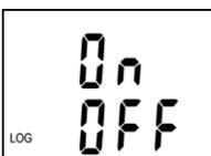
Instrument now displays actual binary state of channel 3 (LCD upper line) and channel 4 (LCD lower line). Symbol On indicates closed contact, symbol OFF indicates open (or not connected) contact.
