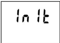
New initialization of logger can occur in switching ON the logger (immediately after displaying of all LCD segments for checking) e.g. after replacement of totally discharged battery for new one. State is indicated by INIT reading. It can be displayed for about 12 s.
