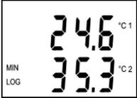
Switched ON logger permanently (with 10 s interval) updates memory of minimum and maximum values of temperature channel 1 and channel 2 (not relevant for binary inputs). If displaying of MIN/MAX values is selected, minimum measured value is displayed at the LCD lower line (indicated by symbol MIN) and then similarly maximum measured value (indicated by symbol MAX).
