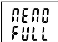
If memory in non-cyclic mode is totally full data logger is switched off and display reading is MEMO FULL. It appears also if logger is operated with switched OFF display.
