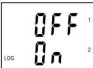
**If LCD display is ON** actual states on binary inputs of channel 1 and channel 2 are displayed. Symbol On indicates closed contact (resp. high voltage level), symbol OFF indicate opened or not-connected contact (resp. low voltage level). Symbol LOG indicates record in progress – if LOG blinks, data memory is occupied more than 90%.
