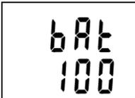
Consequently remaining battery capacity is displayed for about 2 s (value 0 to 100%). It is valid if logger is operated at temperature from -5 to +35°C. If logger is operated often outside of the above temperature range battery life can be reduced to 75%, i.e. if displayed remaining battery capacity drops below 25%, it is recommended to replace the battery.
