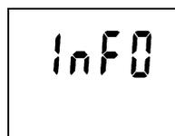
Pressing of ENTER key causes displaying service information on software version (upper LCD line) together with instrument configuration on the LCD lower line.
