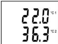
Channel 1 temperature in °C is displayed on the upper LCD line.
