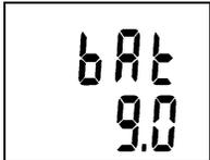
Battery voltage of partially loaded battery is displayed. This value illustrates battery condition.
