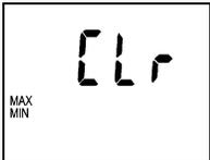
Clearing of minimum and maximum memory of temperature. Memory is cleared after pressing ENTER key. Clearing is confirmed by reading YES on the LCD lower display.
