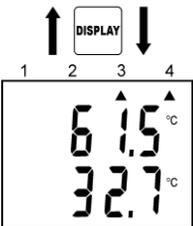
Press DISPLAY key to display the temperature of channel 3 (upper line) and channel 4 (lower line).
