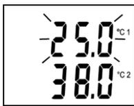
It is possible to set lower and upper limit for each measured temperature. Breaking of the limit is indicated by blinking of the value on the display. Alarm activation can be disabled by setting lower alarm limit up to its maximum. This is indicated by OFF reading at the position of numeric value. Value of upper limit of the same alarm is indifferent.
