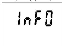
Each pressing of ENTER key causes displaying of service information on software version (upper LCD line) together with instrument configuration on the LCD lower line.
