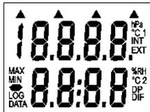
Connect external probe to the instrument before switching ON. The probe is calibrated with the instrument and it is not possible to replace it with another probe from another instrument. Switch ON the instrument by pressing ON/OFF key. After switching ON the instrument all symbols on the LCD are displayed. If the ON/OFF key is being held pressed, all LCD symbols are displayed till the key is released.
