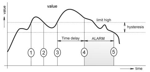
In Point 1 the measured value exceeded the limit. From this time, the time-delay is counting. Because at point 2 the value dropped below the limit value before the time delay expired, alarm was not set.
