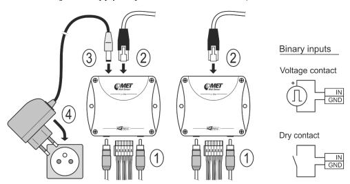
Binary inputs terminals connection procedure:
