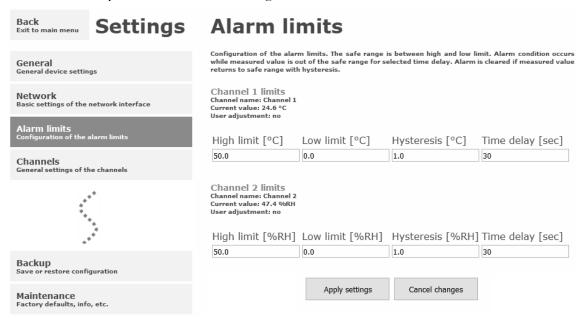
Example of setting the limit to the upper alarm limit:
