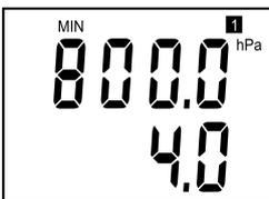
It shows preset value of pressure for current output I1. Lower LCD line shows current value (at mA) which is associated to the lowest pressure output (value displayed at upper LCD line). Here 4 mA corresponds to 800 hPa.
