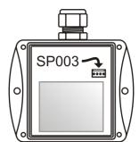
when new setting is saved and finished, disconnect the cable from the device, connect wires into its terminals and place the lid back to the device
