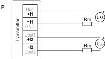
Loop resistance value Rc = Rm + resistance of wires shall fulfill the condition  $Rc[\Omega] < 40 \times Uss[V] - 360$ .
