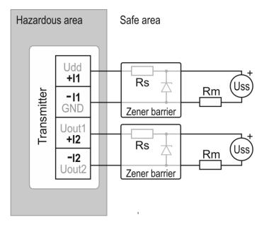
Loop resistance value Rc = Rm + Rs + resistance of wires shall fulfill the condition  $Rc[\Omega] < 40 \times Us[V] - 360$ .
