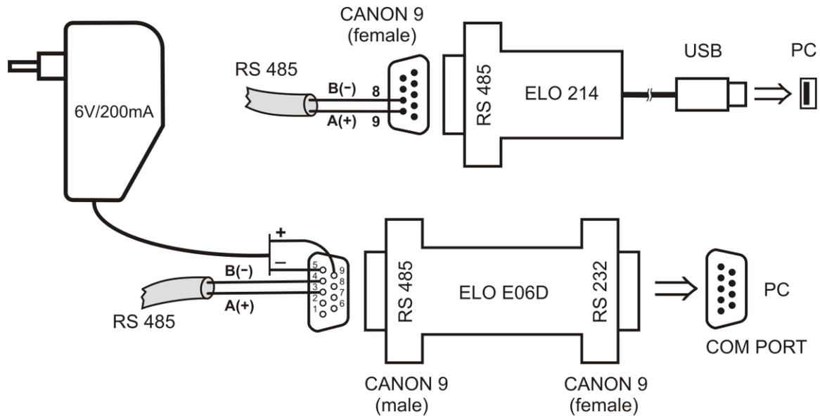
The **ELO E214** converter is an optional accessory for connection of transmitter with RS485 interface to the PC via USB port. Link RS485 is connected across pin 9 A(+) and pin 8 B(-). The pull up, pull down and termination resistors are part of the transmitter. These internal resistors can be connected to the bus by connecting the corresponding pins of CANON connector (for more information see the operation manual for ELO E214).
