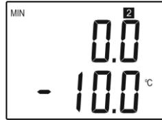
Press the button again to get value of temperature corresponding to output current 4mA (output voltage 0V).
