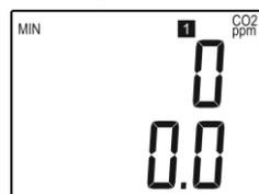
Upper line of the LCD display shows value of CO2 concentration corresponding to output current 4mA (output voltage 0V).
