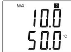
After next pressing of the button LCD shows value of temperature corresponding to output current 20mA (output voltage 10V).
