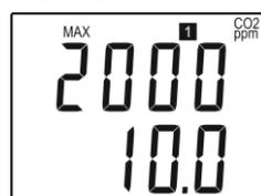
Press the button again and upper line of the LCD display shows value of CO2 concentration corresponding to output current 20mA (output voltage 10V).
