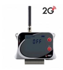
GSM datalogger is designed to record from four binary inputs or from two pulse and two binary inputs. In case of exceeded set limits, SMS and JSON messages can be sent via GPRS data connection. Measured values can be sent to the internet storage <a href="COMET Cloud">COMET Cloud</a>, which is a complete monitoring, alarm and analysis system.
