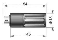
Digital probe with connector MiniDIN, direct insertion.
