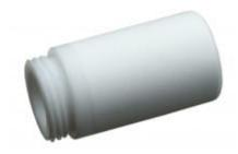
Teflon (PTFE) sensor cover (white color), with increased resistance against splashing water, non-absorbent surface. Filtering ability 25 $\mu$ m. Temperature range -40°C to +125°C.
