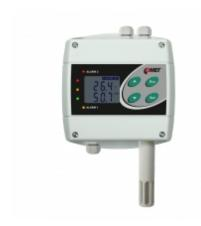
Humidistat, thermostat with two relay outputs. Outdoor, indoor use. Humidistat with built-in humidity, temperature sensors. Measured values are also converted to other humidity interpretation: dew point temperature, absolute humidity, specific humidity, mixing ratio, specific enthalpy.
