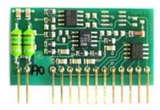
$\label{eq:constraint} \mbox{Accuracy $\pm 0.1\%$ FS. Galvanically unisolated.} \\ \mbox{Two-wire connection.}$
