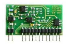
Binary input for potential-less contacts. Maximum resistance of closed contact: 1000 ohms. Minimum duration for recording: 200ms. Galvanically isolated. Galvanic isolation is not designed as safety protection.
