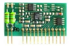
Measuring range -10 to  $+50^{\circ}$ C. Accuracy  $\pm 0.06^{\circ}$ C. Galvanically unisolated. Two-wire connection. Input for precise measurement. Two-wire connection. Only galvanically not isolated version.
