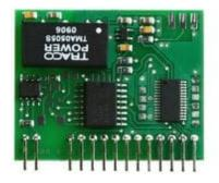
Input for serial signal RS485 for devices supporting Modbus RTU or Advantech protocol. E.g. measurement from Comet Tx41x Hx4xx temperature, humidity, pressure, transmitters. Only devices using same communication protocol and same communication speed can
