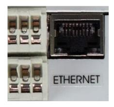
Built-in LAN interface for MS6D, MS6R data logger connection to Ethernet (Internet) network. Communication via: SNMP, SOAP, www pages, Modbus TCP. In case of limits exceeding alarm is activated and warning email or SNMP trap are sent to specified addresses.
