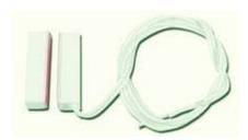
Magnetic door contact, connectable to binary inputs with cable length 2 meters. Plastic body. The dimensions of 49x14x13mm, working distance of 30 mm.
