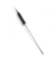
Temperature probe with Ni1000/6180 ppm sensor. Hand held pointed tip probe -30 to 220  $^{\circ}$ C. With 1 meter cable and CINCH connector.
