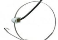
Temperature probe with Pt1000 sensor. Surface probe for tubing and flat surface, range from -30 to  $+130^{\circ}$ C, 5 meters cable, IP65. With ELKA connector.
