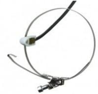
Temperature probe with Pt1000 sensor. Surface probe for tubing and flat surface, range from -30 to  $+130^{\circ}$ C, 5 meters cable, IP65. With CINCH connector.
