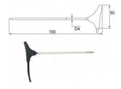
Temperature probe with Pt1000 sensor.
