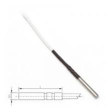
Multi-purpose watertight IP67 probe -190 to +150°C. Accuracy class B. Stainless steel 17240 with teflon cable of specified length, with ELKA connector. Diameter 5  $\pm$  0.1 mm, length 50mm.
