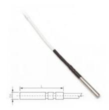
Multi-purpose watertight IP67 probe -190 to  $+150^{\circ}$ C. Accuracy class B. Stainless steel 17240 with teflon cable of specified length, with MiniDin connector. Diameter 5  $\pm$  0.1 mm, length 50mm.
