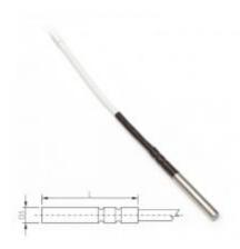
Multi-purpose watertight IP67 probe -190 to  $+150^{\circ}$ C. Accuracy class B. Stainless steel 17240 with teflon cable of specified length, with ELKA connector. Diameter 5  $\pm$  0.1 mm, length 50mm.
