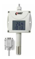
Ambient thermometer hygrometer barometer. Outdoor, indoor use. Built-in relative humidity, temperature, atmospheric pressure sensors. Measured values are also converted to other humidity interpretation: dew point temperature, absolute humidity, specific humidity, mixing ratio, specific enthalpy.
