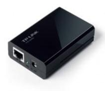
TL-POE10R Power over Ethernet (PoE) splitter supplied by TP-Link company. This adapter is necessary for powering Ethernet transmitters or Multiloggers from PoE switch. It is necessary to select proper output voltage by a switch: 12V for Txxxx transmitters, 5V for Multilogger!!!
