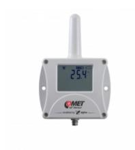
The device measures the temperature from an external Pt1000 probe on the cable - you can choose it from an optional accessory.
