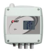
The W0941 sensor with LoRaWAN network output measures temperature from four external Pt1000 probes on the cable and can be installed directly in the measured environment thanks to its IP65-rated enclosure. LoRa devices are powered by a replaceable battery with a lifespan of up to 10 years (3 years standard). External power with optional accessories is also available.
