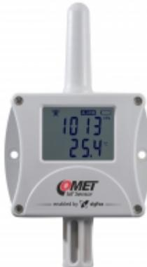
The device measures the temperature, humidity and atmospheric pressure from the built-in internal sensors. It is characterized by a simple compact design with the possibility of installation directly into the measured space. The sensor can be used [with a suitable sensor cap](#) even in more demanding conditions.
