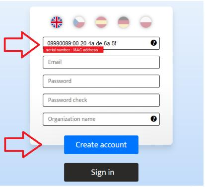
3. After the device is registered into COMET Cloud using serial number and MAC address, it needs to be determined SOAP server address. Address can be determined at list of devices (My Devices) and option How to configurate a web sensor to send data to COMET Cloud accessible via left mouse click.
