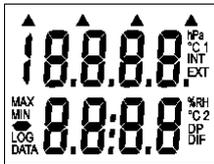
Connect the external probe to the connector before switching ON the instrument. Probe is calibrated with the delivered instrument and it is not possible to replace it with another (if you have several instruments of this type). Switch ON the instrument by pressing ON/OFF key. After switching ON the instrument all symbols on the LCD are displayed. If the ON/OFF key is being held pressed, all LCD symbols are displayed till the key is released.
