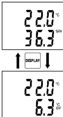
Temperature is displayed on the upper LCD line and relative humidity in %RH is displayed on the lower LCD line.
