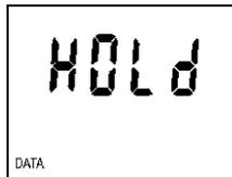
Press ENTER key to display values stored in the HOLD memory. Press DISPLAY key to display other stored values. Press ENTER key to leave this mode.
