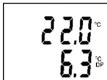
Temperature in °C is displayed on the upper LCD line and relative humidity in %RH is displayed on the lower LCD line.
