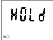
Press ENTER key to display values stored in the HOLD memory. Press DISPLAY key to display other stored values. Press ENTER key to leave this mode.
