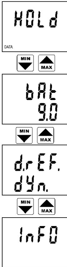
Press ENTER key to display values stored in the HOLD memory. Press DISPLAY key to display other stored values. Press MENU key to leave this mode.
