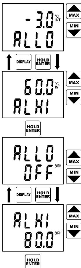
Reading ALLO indicates adjusted lower alarm limit (here air temperature). Set the desired value by means of the arrow keys. Press and hold the arrow key UP to make value increase fast. Press and hold the arrow key DOWN to make value decrease fast. Release the arrow key and press ENTER to confirm new limit.
