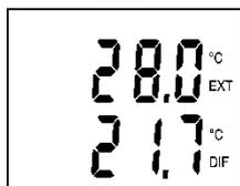
Press DISPLAY key to display other readings - external probe temperature in °C (symbol EXT) and difference between external temperature and dew point temperature (symbol DIF). The difference is defined as  $t_{dif} = t_{ext} - t_{dp}$
