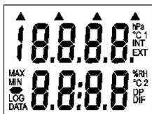
If you wish to use the external temperature probe, connect it before instrument switching ON. Switch ON the instrument by pressing ON/OFF key. After switching ON the instrument all symbols on the LCD are displayed. If the ON/OFF key is being held pressed, all LCD symbols are displayed till the key is released.
