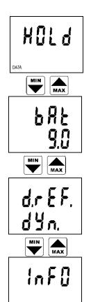
Press ENTER key to display values stored in the HOLD memory. Press DISPLAY key to display other stored values. Press ENTER key to leave this mode.
