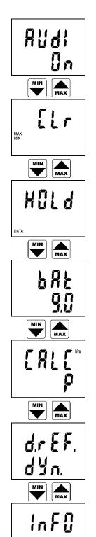
This item indicates if audio signaling of alarm indication is switched on (On) or switched off (OFF). Press ENTER key to change actual setting. Notice: if the battery voltage is low, audio indication is out of operation to reduce current consumption independently on this selection.
