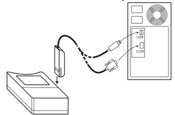
After connecting the logger to the computer reading of logger info is enabled by means of the PC software and also setting of the instrument accordingly to the user needs (menu *Configuration / Setting of instrument parameters*). Before logging start it is necessary:
