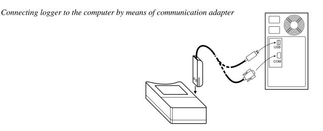
Notice: USB connector can be located also from the computer front side
