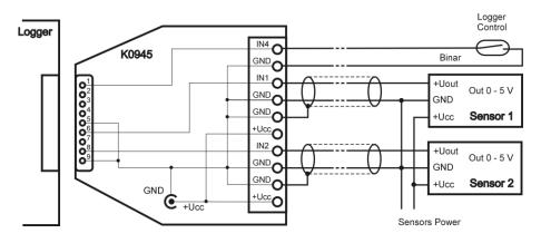
Connection to sensor signals. Power supply is located near the sensor:
